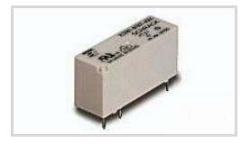
Power Relay Type: **Standard** Coil Magnetic System: **Monostable, DC** Coil Power Rating Class: **200 – 300 mW** Coil Power Rating DC: **221 mW** Coil Resistance: **652 Ω**
