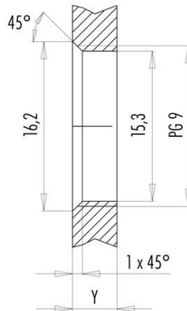
Installation direction: o-ring sits on chamfer.
