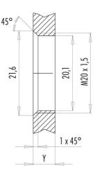
Installation direction: o-ring sits on chamfer.
