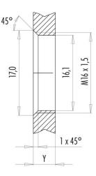
Installation direction: o-ring sits on chamfer.
