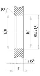
Installation direction: o-ring sits on chamfer.
