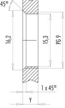
Installation direction: o-ring sits on chamfer.
