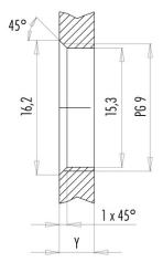
Installation direction: o-ring sits on chamfer.
