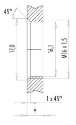
Installation direction: o-ring sits on chamfer.
