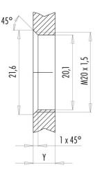
Installation direction: o-ring sits on chamfer.
