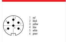
Contact arrangement (Plug-in side)
