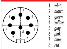
Contact arrangement (Plug-in side)
