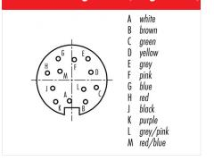
Contact arrangement (Plug-in side)
