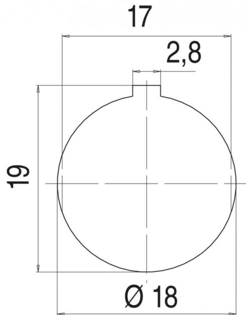
Product description      **M16 IP40 male panel mount connector, Contacts: 8 DIN, unshielded, solder, IP40, front mounting**
