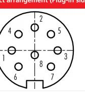
5 A 60 V 500 V 1 Т Ш  $\geq 10^{10} \Omega$ unshielded IP68 IP67 > 500 Mating cycles
