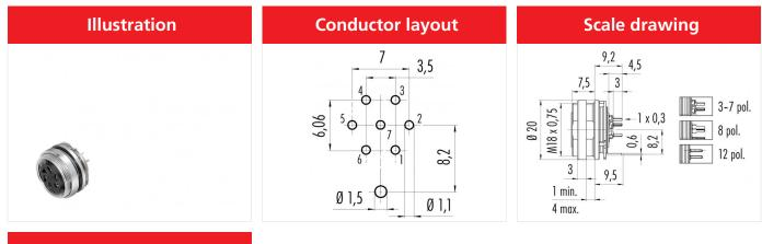
Contact arrangement (Plug-in side)
