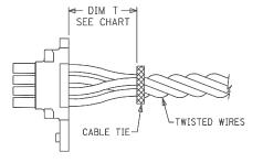
The "T" dimension defines a "free" length of wire, or a length of wire that is not subject to significant bias by external factors such as a wire tie, wire twisting, or other means of bending or deforming of the wires that repositions them from their natural relaxed state or location where they enter the housing. Wires are to be dressed in such a manner to allow the terminals to float freely in the pocket.
