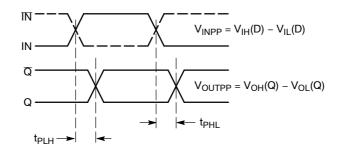
Figure 19. AC Reference Measurement
