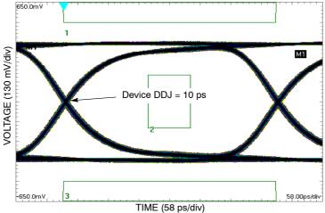
Figure 2. Typical Output Waveform at 2.488 Gb/s with PRBS  $2^{23-1}$  (V<sub>INPP</sub> = 400 mV; Input Signal DDJ = 14 ps)
