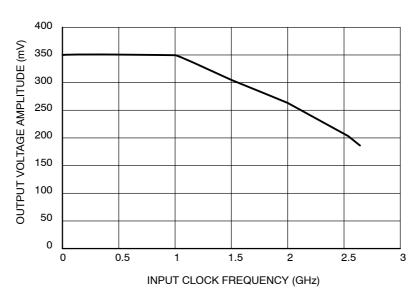
Figure 4. Output Voltage Amplitude ( $V_{OUTPP}$ ) versus Input Clock Frequency ( $f_{in}$ ) and Temperature (@  $V_{CC}$  = 2.5 V)
