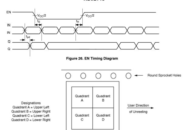
Figure 27. Tape and Reel Pin 1 Quadrant Orientation
