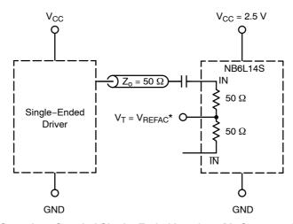
Figure 18. Capacitor-Coupled Single-Ended Interface (V<sub>T</sub> Connected to V<sub>REFAC</sub>)
