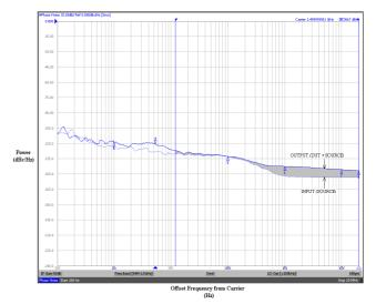
Figure 8. Typical Phase Noise Plot at  $f_{carrier} = 1.5 \text{ GHz}$
