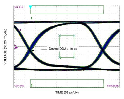
Figure 9. Typical Output Waveform at 2.488 Gb/s with PRBS  $2^{23-1}$  and OC48 mask ( $V_{INPP} = 100$  mV; Input Signal DDJ = 14 ps)
